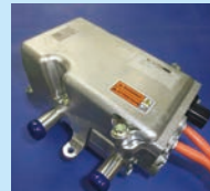
Hot Water Heater
